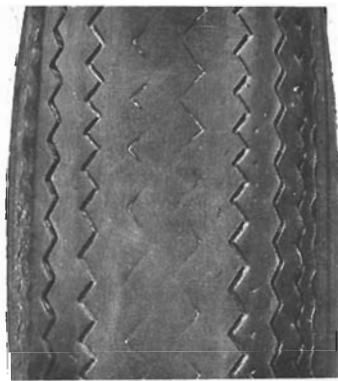
Fig. 13-8. Overinflation wear. Tire worn out by running it with excessive air pressure.
