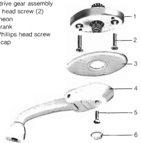
Fig. 8-3. Components of hand crank and cable drive gear.
