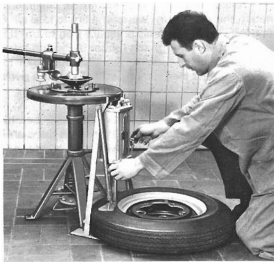
Fig. 13-3. Pressing tire bead off rim.
