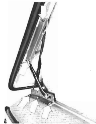
Fig. 7-39. Bolts (lower three arrows) and self-locking nuts (upper two arrows).
