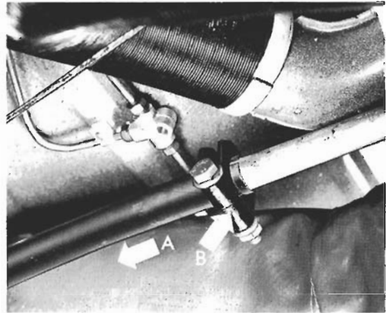
Fig. 13-7. Front selecting rod being pushed forward (arrow A) before clamp (arrow B) is tightened.
