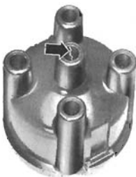
Fig. 3-2. Typical carbon tracks in distributor cap.
