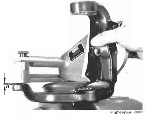
Fig. 6-9. Special gauge in position with its center plate slipped over the stub axle. Check the steering arm at a , as described in the text.
