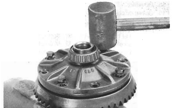
Fig. 11-4. Rubber mallet being used against bolt heads to drive off ring gear.
