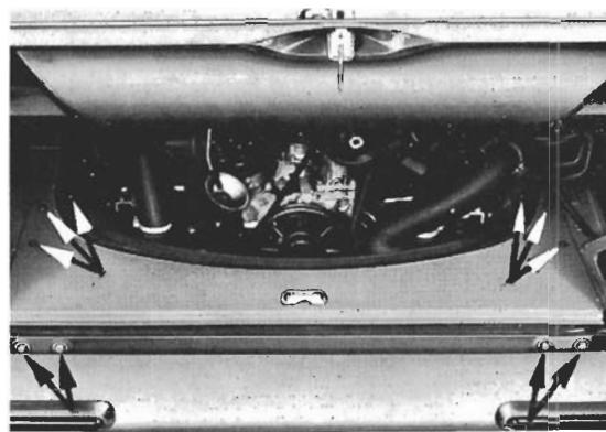
Fig. 3-1. Screws (arrows) that hold the rear engine compartment panel.
