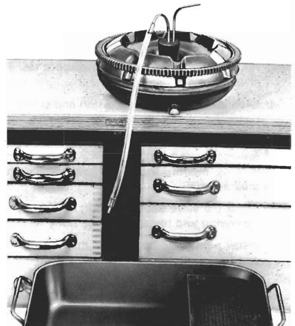
Fig. 8-3. Siphon and oil receptacle in position.
