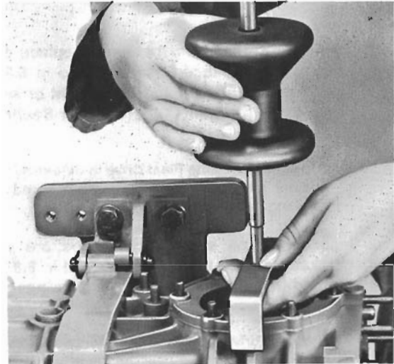
Fig. 6-3. A slide hammer and puller being used to remove a side cover from an early transmission.
