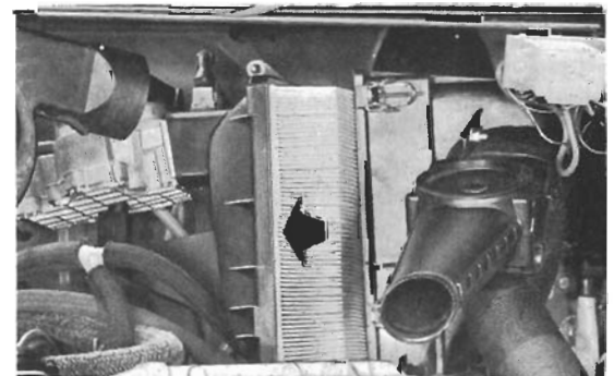
Fig. 6-2. Preparation for filter removal. Push air cleaner body to left (arrow).
