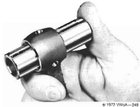
Fig. 18-2. Piston pin fit being checked. The pin should be a push fit in a new bushing.
