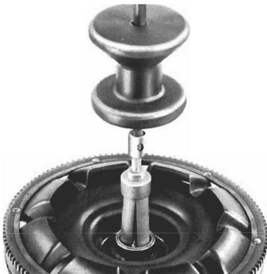
Fig. 8-1. Extracting converter bushing. Use clean tools to keep dirt out of converter.
