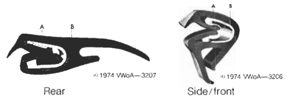
Fig. 7-35. Cross section of rear seal (left); cross section of front and side seals (right). The rubber seals are at B ; the steel clips at A .
