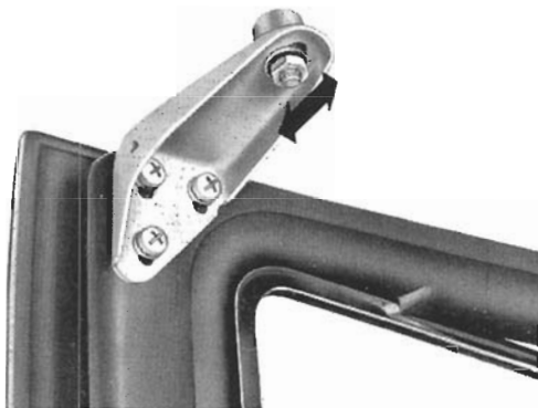
Fig. 5-39. Top roller adjustment. Position the roller on the bracket as needed (arrows) to align the door with the body.
