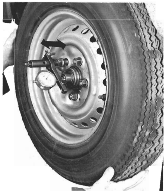
Fig. 5-13. Checking front wheel bearing axial play.
