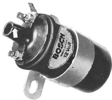
Fig. 3-3. Typical carbon track on coil tower.
