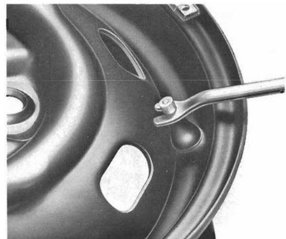
Fig. 13-5. A valve tool being used to install a new valve in the rim.
