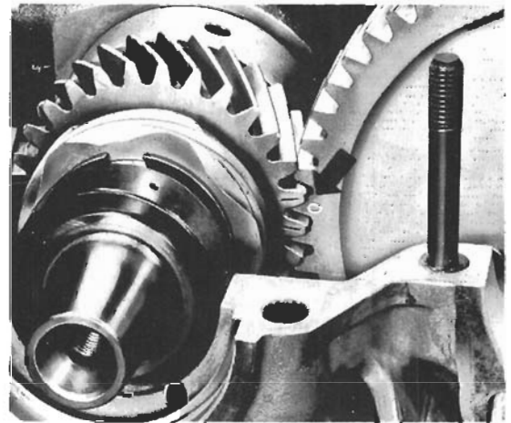
Fig. 17-4. Camshaft installation. The tooth marked with a small circle (arrow) goes between the two marked teeth on the crankshaft gear.
