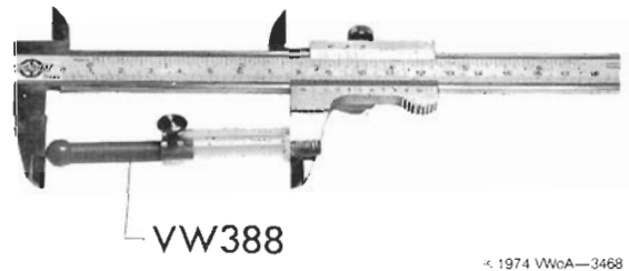
Fig. 12-10. Vernier caliper being used to adjust measuring bar VW 388 to as near 80.00 mm as possible.
