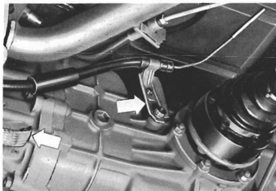
Fig. 4-12. Angled support bracket for clutch cable guide tube (right arrow). Upper mounting nut has been removed. Also disconnect the ground strap indicated by the left arrow.
