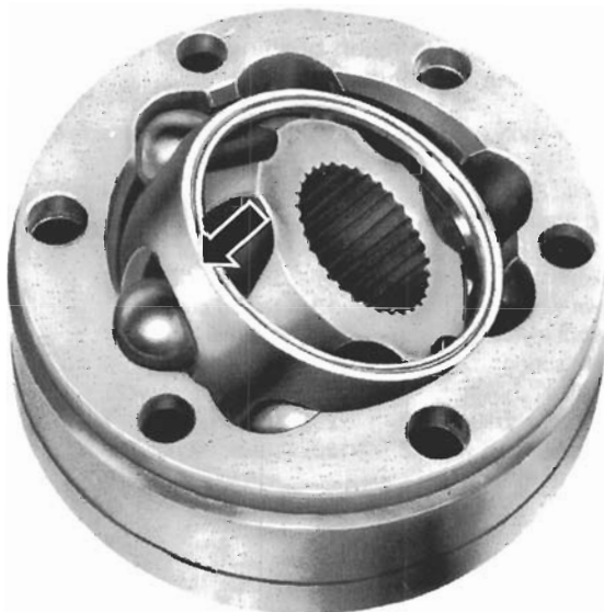
Fig. 3-12. Balls being engaged in the grooves of the outer ring. Apply hand pressure at the point indicated by the arrow.
