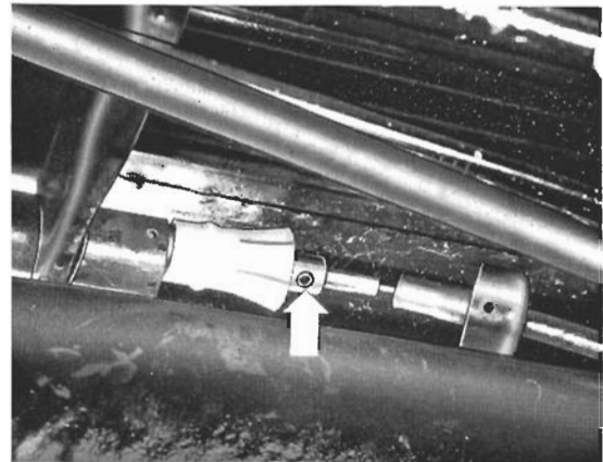
Fig. 13-4. Spring pin (arrow) that holds the cable on the rear selecting rod.
