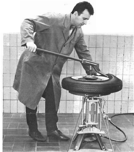
Fig. 13-4. Prying tire sidewalls over rim edges.
