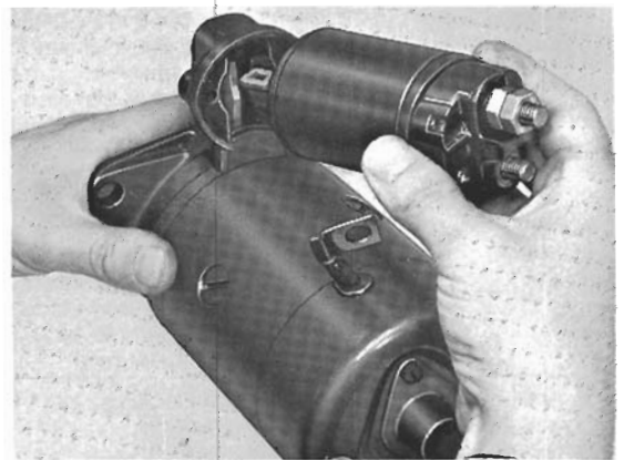
Fig. 5-2. Solenoid being installed. Hook pull rod eye over engaging lever. Use sealing compound between solenoid end face and drive end plate.
