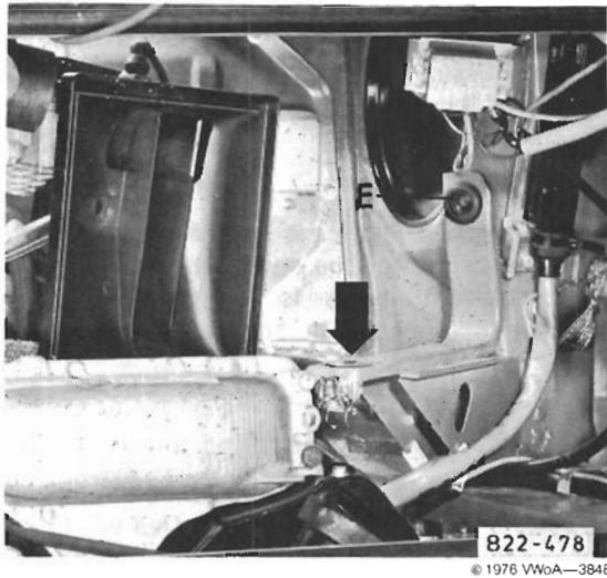
Fig. 6-3. Mountings for air cleaner cover. Rubber grommet is at E; clamp engagement point is at arrow.
