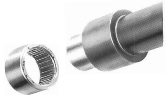
Fig. 8-5. Correct relationship of bearing to driving tool.
