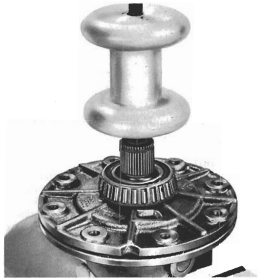
Fig. 6-9. Differential housing cover being removed by lifting the short gearshaft with a slide hammer.
