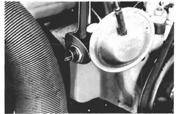
Fig. 9-3. Oil pressure switch being removed from single-carburetor engine. See Fig. 9-1 for the switch location on the dual-carburetor and fuel injection engines.
