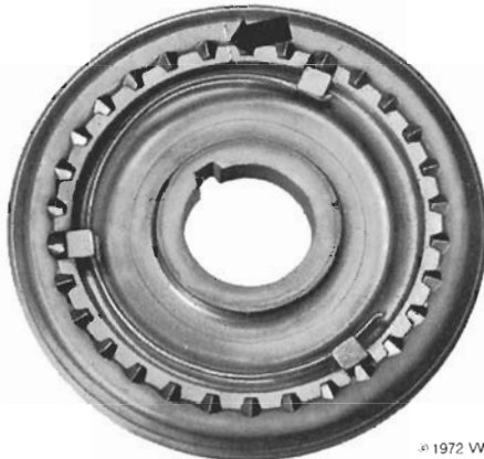
Fig. 7-29. Alignment marks (arrow).
