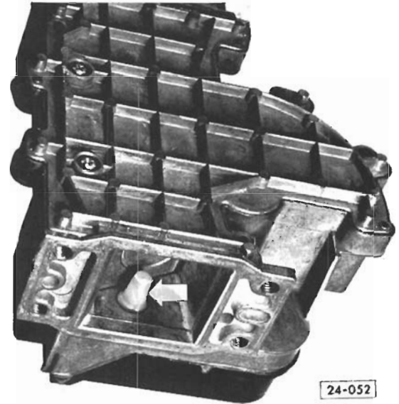
Fig. 4-15. Location of temperature sensor I (arrow).
