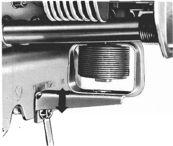
Fig. 6-5. Bracket movement (double arrow) that permits thermostat to be adjusted.
