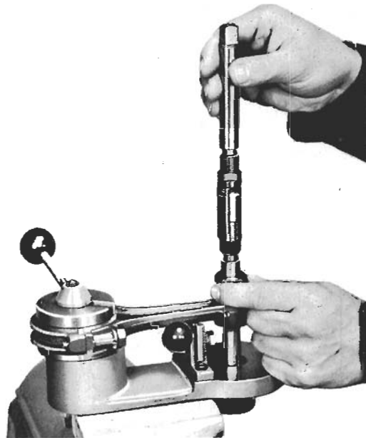
Fig. 18-8. New bushing being reamed. Afterward, using the piston pin, recheck rod alignment.
