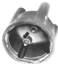
Fig. 3-2. Typical carbon tracks in distributor cap.
