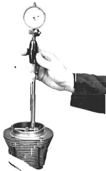
Fig. 13-7. Cylinder bore being measured with special dial indicator.
