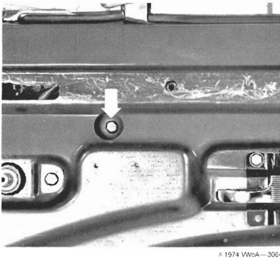
Fig. 5-24. Opening (arrow) for access to guide channel bolt.
