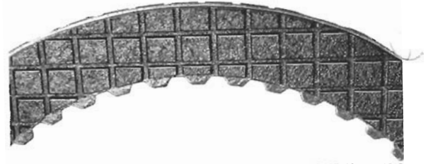
Fig. 10-16. Direct and reverse clutch lined plate. The waffled surface of the lining distinguishes these plates from those of the forward clutch.
