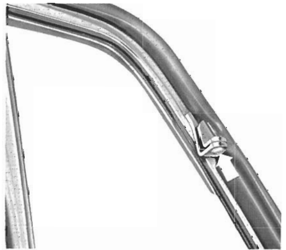
Fig. 5-27. Rivet that holds the vent wing to the vent wing frame. Grind the end off the rivet at the point indicated by the arrow.
