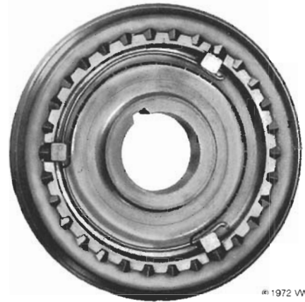
Fig. 7-30. Positions for the spring rings. Make sure the spring ring ends are fully hooked over the synchronizer keys.
