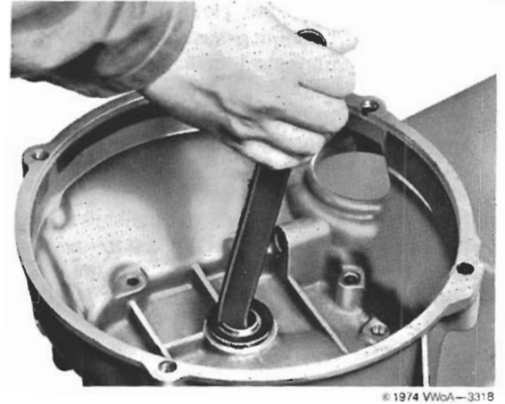
Fig. 5-3. A hook-type tool being used to remove the rear driveshaft oil seal. Be careful not to damage the seal recess in the housing or the oil return sleeve that is behind the seal.
