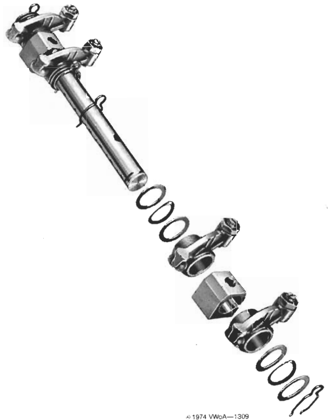
Fig. 10-5. Exploded view of single-carburetor engine rocker arm shaft assembly. Replace worn or corroded washers and end clips.
