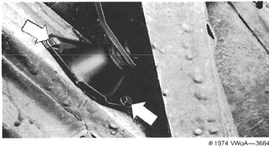
Fig. 15-15. Bolts (arrows) that hold the pedal assembly on the vehicle frame.
