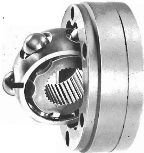
Fig. 3-8. Ball cage and ball hub being separated from outer ring. Position the ball hub and ball cage perpendicular to the outer ring, then push in the direction indicated by the arrow.
