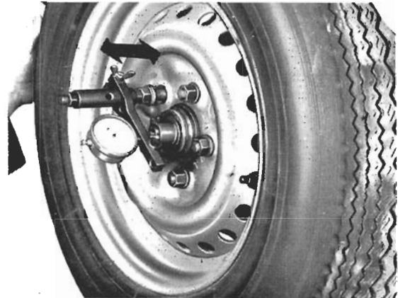
Fig. 5-2. Dial indicator being used to measure wheel bearing axial play (indicated by arrow).
