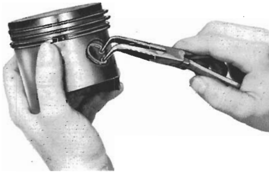
Fig. 13-2. Piston pin circlip being removed or installed.
